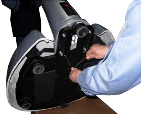
Pic #5 Tighten the column to the base
